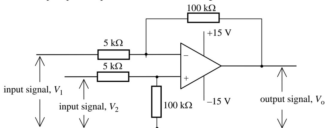
The op-amp has two inputs,  $V_1$  and  $V_2$ . The voltage applied to  $V_1$  is 0.4 V and the voltage applied to  $V_2$  is 0.5 V. Calculate the output from this op-amp. (2)
